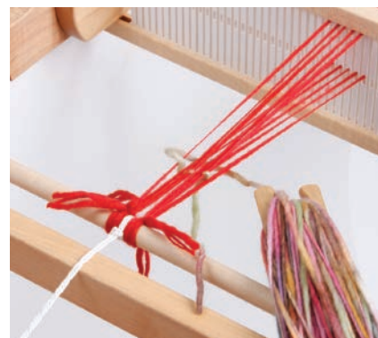
b. Change the shed without bringing the rigid heddle forward. Take the shuttle under the warp and back to the side where it previously entered.
