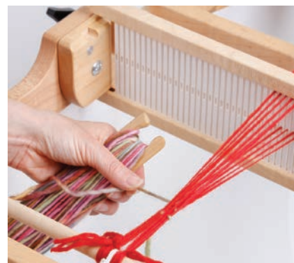
c. Pass the shuttle through the open shed and then gently tug downward on the weft to tighten.
