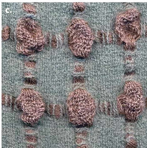
a. In the fullled sample, design squares are shorter than they are wide. b. The first scarf was woven with design squares taller than wide. c. The result after fulling was design squares taller than they are wide. More shrinkage occurred in the direction of the smallest measurement.
