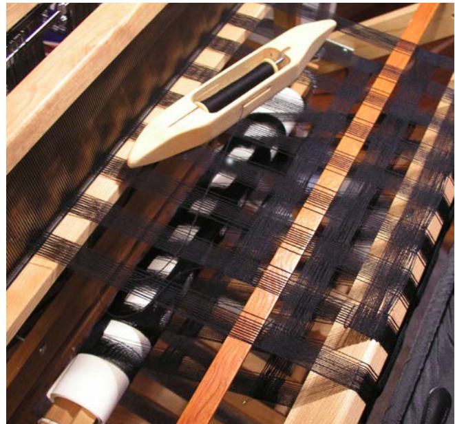
a. A wooden spacer is inserted after each section of 19 picks of plain weave. The spacer is removed and reinserted as needed. Plain-weave sections using shafts 1 and 2 alternate with plain-weave sections using shafts 3 and 4 to appear as if the sections weave with each other.
