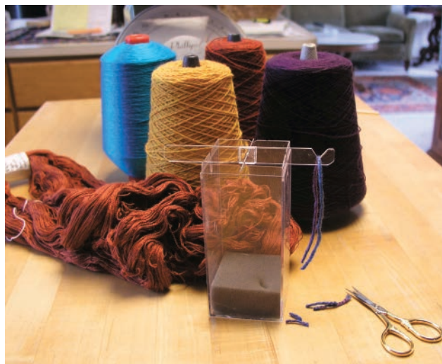
b. Trim off small pieces of the yarn until the balance swings to become horizontal.
