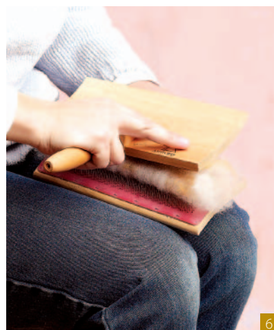
Use the edge of the right carder and your left hand to start rolling the rolag.
