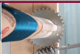
Easy warp control with the cog wheel system
