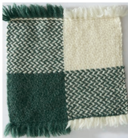
FROM LEFT TO RIGHT: Sample 1 is lightly fullled Erin sett at 8 epi, Sample 2 is moderately fullled Erin sett at 8 epi, and Sample 3 is felted Erin sett at 8 epi.
