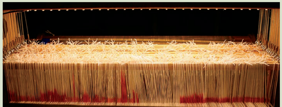
Extra light helps avoid threading mistakes. PHOTOS BY TIEN CHIU
