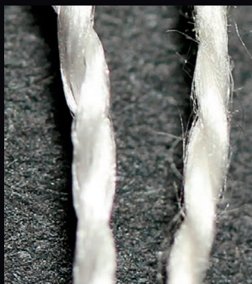
Reeled silk on the left (NS-18K from Habu) and spun silk on the right (30/2 silk from Mint Fabrics, India). Note the smooth texture of the reeled silk vs. the fuzzy surface of the spun silk.
