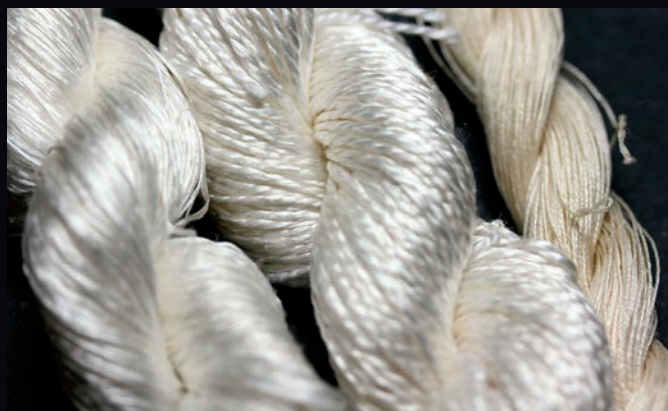
Left: loose-twist tram; middle: a light sportweight yarn designed to simulate an old yarn called “purse twist”; right: raw (in the gum) size C sewing thread.
