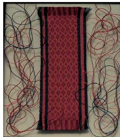
An 8-shaft warp-faced compound tabby weave in 60/2 silk that was sett at 96 EPI. 6" x 2½". PHOTO BY EMORY SOMMERS
