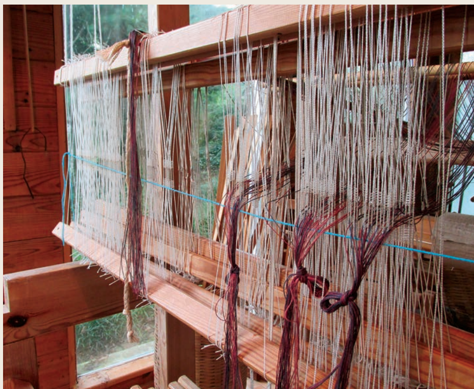
A guide thread keeps fine warp threads visible and tidy at the front of the shafts.
