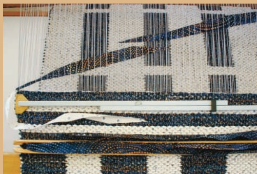
A temple helps keep an even width and good selvages. See Resources for more information on using a temple. BEVERLY WEAVER
