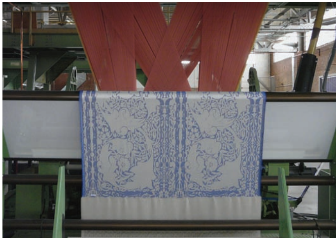
One of the mill's Jacquard looms at work weaving a damask coverlet fabric.
