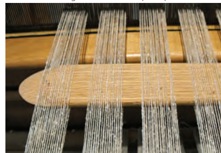
d. The stick is turned on edge to insert the shuttle.
