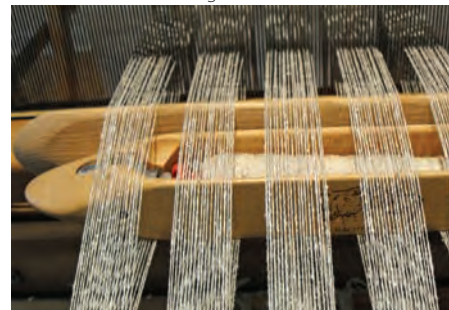
d. The stick is turned on edge to insert the shuttle.
