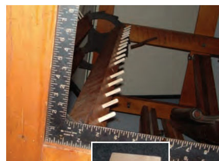
Right-angle joints should measure 90 degrees. Wooden mallet is used to tighten frame joints.
