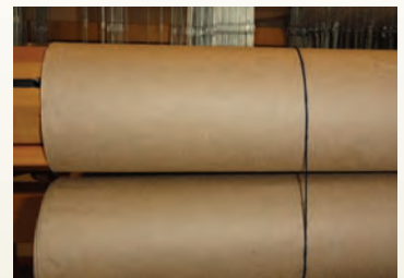
String tied around paper used between layers of warp keeps the paper tidy.
