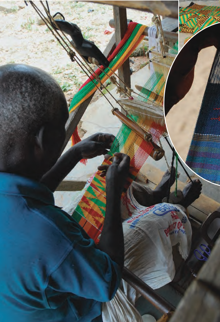
Kyere Badu weaves on his porch in Bonwire. Carved wooden pulleys support two sets of heddles, one for plain weave, one for pattern, that are manipulated with the feet.
