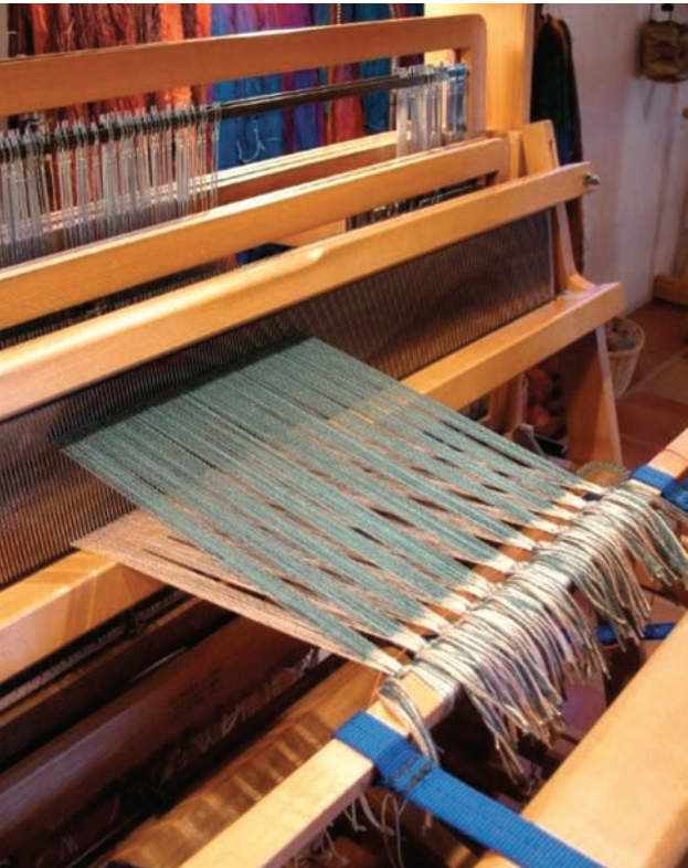
Because there are two layers of cloth, doubleweave is sett at twice the density of a single layer, making it especially important to provide a clean shed.
