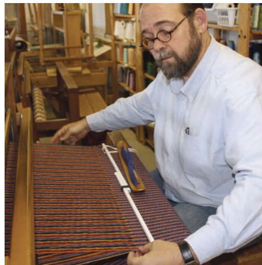
Using a temple for doublewidth weaving helps prevent the crowding of the warp threads at the fold and allows you to pull the weft snugly there; see page 21.
