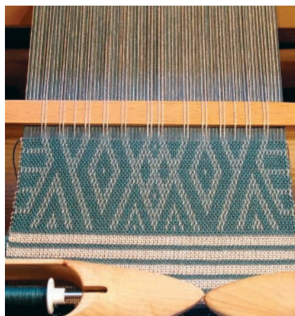
At left: Use a reed that gives four ends per dent at the chosen sett, so it will be easy both to see mistakes and to count warp pairs for doubleweave pick-up. At right: You can create elaborate doubleweave patterning with simple tools.
