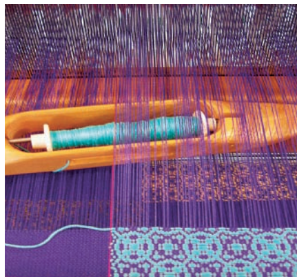
Enter the pattern shuttle under the guide string and all of the raised threads between guide strings. Take the shuttle out under the guide string on the opposite side. Weave a tabby pick and repeat.
