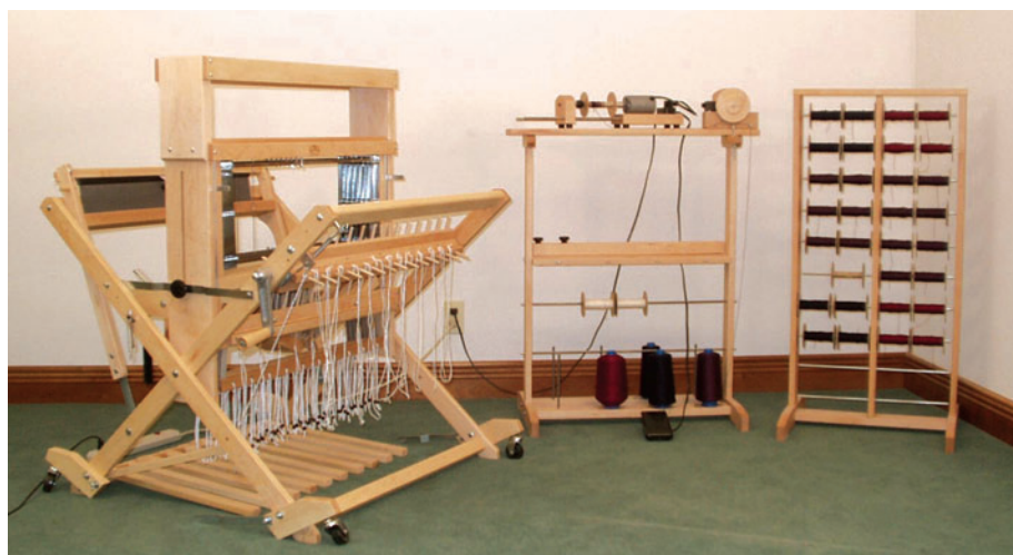
Sectional warping equipment: a sectional warp beam, a cone holder (optional), a bobbin winder for winding the spools (either electric or manual), a yardage counter (to the right of the bobbin winder above), and a spool rack. You'll also need a tension box; see page 71.
