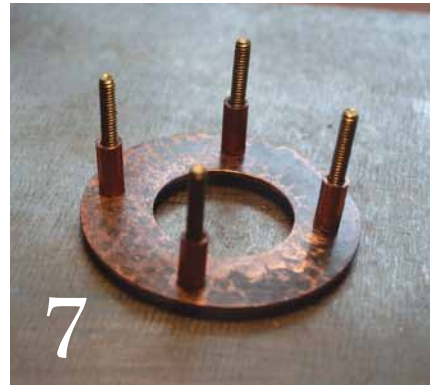
PHOTO 7: Slide a riser on each of the 4 screws, being careful not to damage threads.
