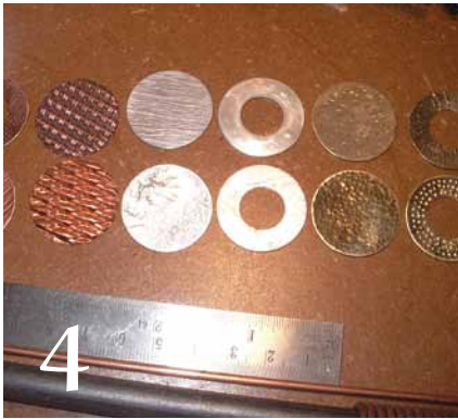
PHOTO 4: Bring each of 12 drilled circles to desired finish by sanding and polishing or tumbling. Patina as desired.
