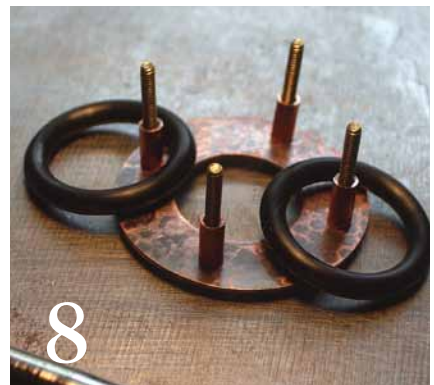
PHOTO 9: Place lower circle onto screws, being careful not to damage threads. Ensure textured side is facing desired direction and O-rings are circling correct risers.
